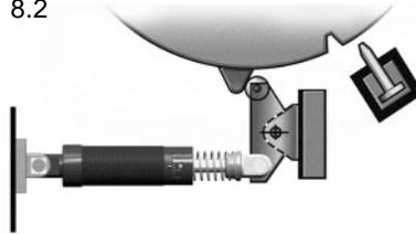
8.1 The latch absorbs the kinetic energy so that the object contacts the fixed stop gently.
