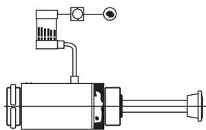
1. The piston rod is immediately returned to its extended position after completing the stroke.
