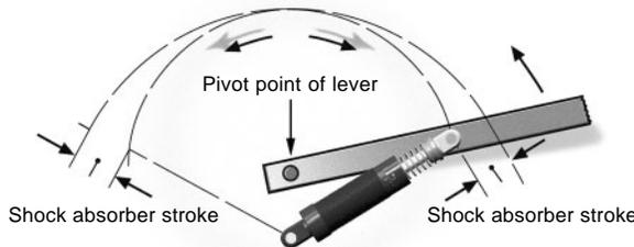
It is possible to use only one shock absorber for both end positions by using different pivot points as shown.
