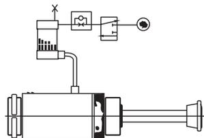
2. The piston rod remains in its retracted position until it is signaled to return. Special bleed-down type check valve is required for this circuit.
