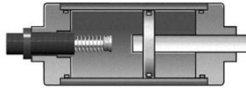
With heavy loads or high velocities normal cylinder cushions are often overloaded. This causes shock loading leading to premature cylinder failure or excessive maintenance. Using oversized cylinders to withstand this shock loading is not the best solution since this considerably increases air consumption and costs.
