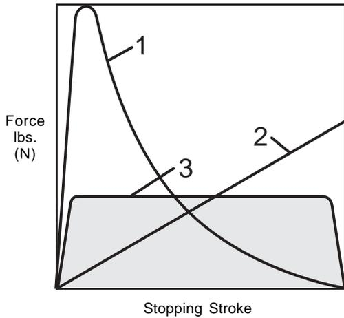
**1. Cylinder Cushions and Dashpots (High stopping force at start of the stroke).**
