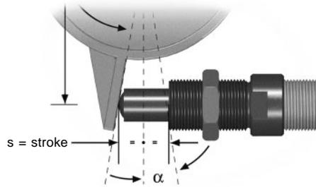
The side loading is removed from the shock absorber piston rod leading to considerably longer life. Wherever possible mount shock absorber so that impacting face is perpendicular to shock absorber axis half way through stroke. See pages 48 and 49 for more details.
