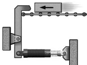
By means of a lever the effective stroke length can be increased and mounting space to the left reduced.
