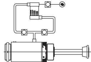
3. A recirculating cooling circuit allows warm oil to return to the tank while cool oil refills the shock absorber. A recirculating cooling circuit substantially increases the shock absorber's hourly energy capacity.
