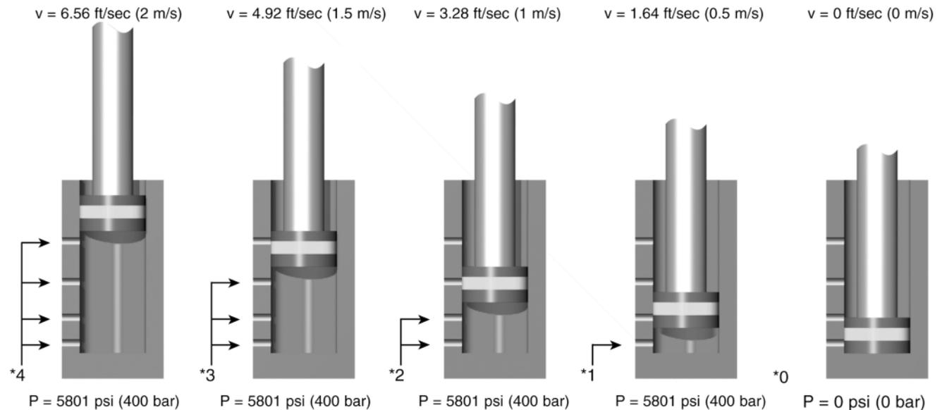
\* As a moving load impacts the shock absorber, the piston travels through stroke and forces hydraulic fluid through the multi-orifice inner tube. The total orifice area decreases at a rate consistent with the decay of impact velocity, resulting in true linear deceleration.
