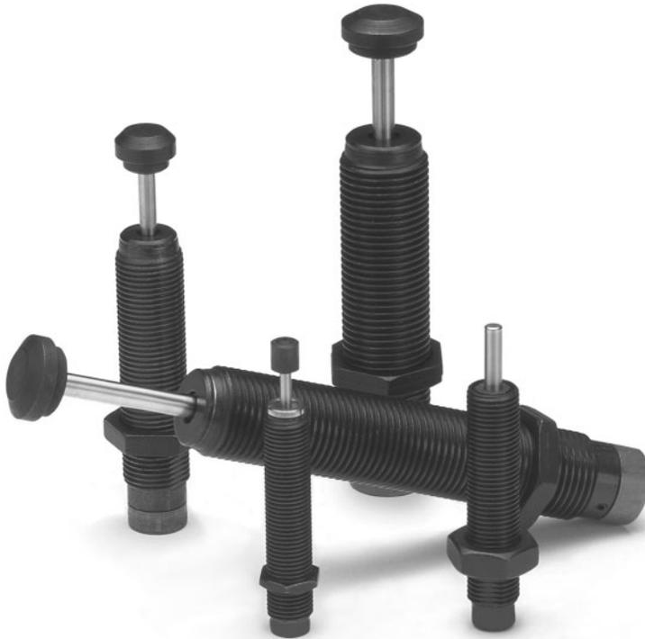
**MA Series miniature shock absorbers** offer a compact design with true linear deceleration, and are adjustable over a wide range of conditions. If your preference is a fully adjustable shock absorber rather than a self-compensating model on your application, then the MA Series provides a directly interchangeable alternative.
