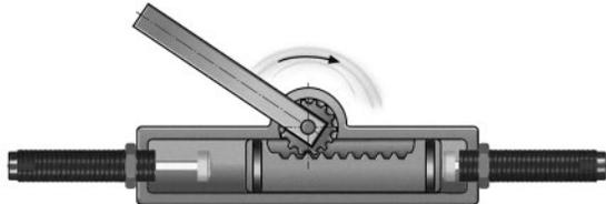
The use of shock absorbers allows higher operating speeds and weights as well as protecting the drive mechanism and housing from shock loads.
