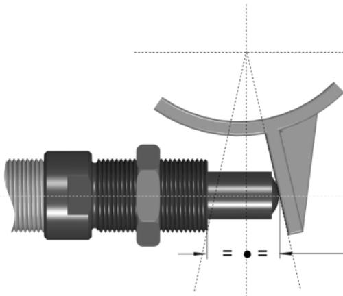
**Problem:** Rotary motion of the striking surface creates side load, which develops a bending moment on the piston rod. This can bend the rod in some cases. In all cases, side load will reduce seal and bearing life.
