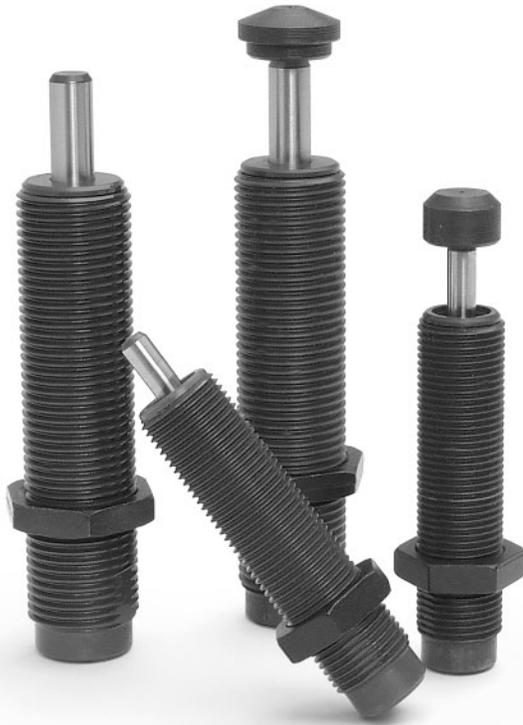
**SC<sup>2</sup> 300 and SC<sup>2</sup> 650 Heavyweight Series Shock Absorbers** deliver up to **950% of the effective weight capacity** and **280% of the energy absorption capability** of standard models. These durable units are ideal for decelerating heavy weights moving at low velocities. The Heavyweight Series design combines the piston and the inner tube into a single component, the piston tube. It acts as both the pressure creating and pressure controlling device.
