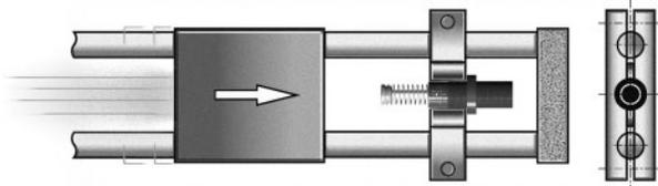
The gentle deceleration of shock absorbers makes the use of adjustable stop clamps possible and removes any chance of the clamp slipping. The kinetic energy is completely removed before the mechanical stop is reached thus making high index speeds possible.
