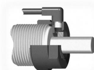
By using this air bleed collar the operating lifetime of shock absorbers in aggressive environments can be considerably increased. The adapter protects the shock absorber seals from cutting fluids, cleaning agents, cooking oils etc. by using a low pressure air bleed.
