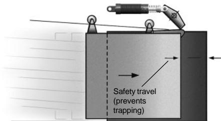
The fire door travels quickly until it reaches the lever. It is then gently decelerated by the lever mounted shock absorber and closes without shock or danger to personnel.
