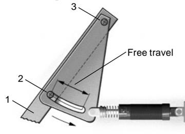
The lever 1 swings with the pin 2 in a slotted hole around pivot point 3. The lever is smoothly decelerated at the extreme end of its travel.
