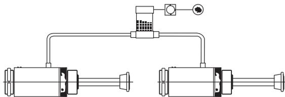
4. When connecting more than one shock absorber to an Air-Oil Tank, use caution in selecting the proper reservoir capacity. For two shock absorbers, the next largest Air-Oil Tank Size is usually adequate.
